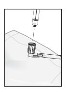
The outside diameter of the syringe needle should not be larger than 22 gauge (0.028 inch).
